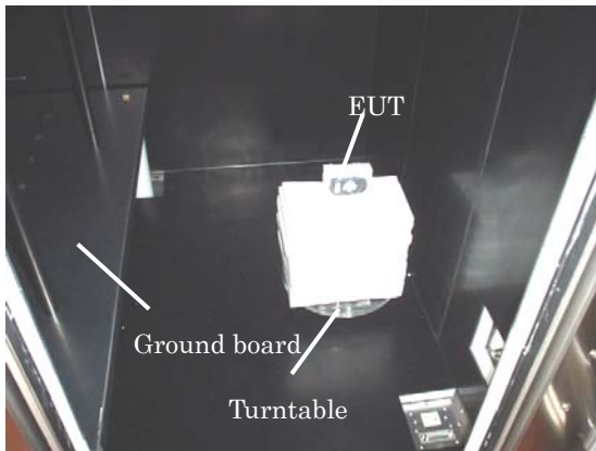
Photo 1 Installation of EUT (keyless entry)
