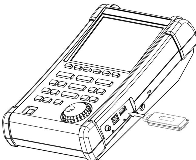
※ If the USB memory is installed again after it is installed once and then removed, the MSA500 series cannot normally recognize it. In that case refer to the following operation.
