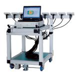
This is a system for measuring the strength of radio wave emitted from DSRC antenna ME9301 (electric field strength).
