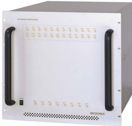
24 × 8 RF matrix switch box MM6824 / 6824C
