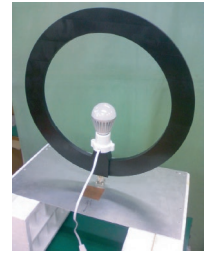
Radiated Emission Measurement of LED Lighting
