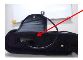
It is possible to operate the USB device because the voltage of 5VDC is always outputted to USB connector(Atype)of MSA400.
