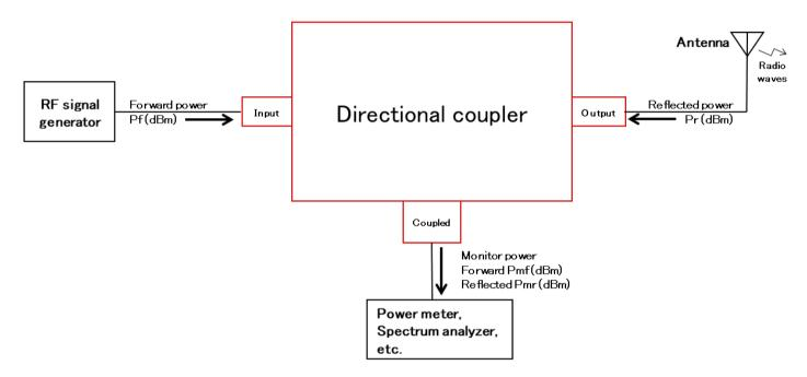
The main specifications of a directional coupler are Coupling : C (dB) and Directivity : D (dB).
