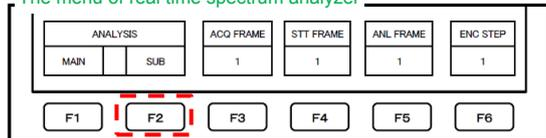
(1) Select "F2" in the menu of real time spectrum analyzer.
