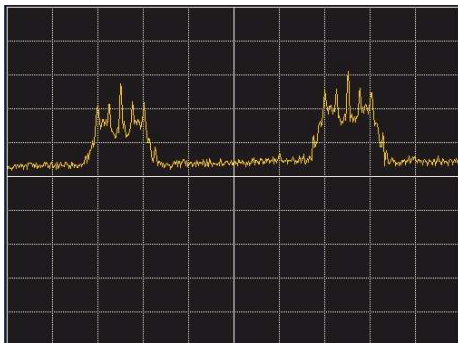
※ 2 channel signals of ETC roadside unit (5795 & 5805MHz)
