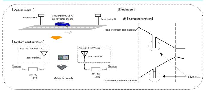
Since mobile phone goes away from the base station A, the receiving level becomes low gradually, and conversely it becomes high gradually in the base station B. Moreover, there may be an obstacle blocking the radio wave in the middle.
