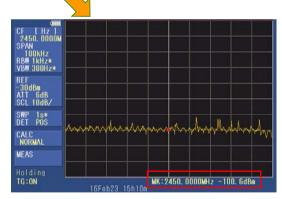
In the connection example, when opening the door: -38.7dBm @ 2450 MHz, but when the door is closed: -100.6dBm @ 2450MHz. However, the measured value of "-100.6dBm" which is the reference value is important. It is judged that the shielding performance deteriorates if the electric field strength level goes upper than this reference value.
