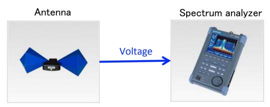
Convert Electric field strength to voltage (Conversion factor = Antenna factor)
